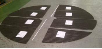
Mats produced to a drawing or template are supplied to a finished size, as requested, and indicated on the "Matting order confirmation form" and should require minimal site adjustment. The mats should then be laid so that the pedestrians walk across the mat ribs, the direction of traffic (DOT), and not along them.
